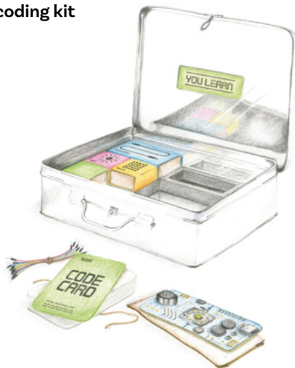
Figure 3. Children's coding kit. Stainless steel case containing 'Your Voice' developers board, various electronic components, and a deck of coding cards. 2025, Pete Thomas.
